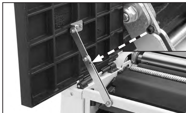
Figure 26. Outfeed table lock arm.
